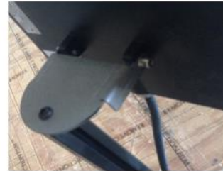
DETAIL 1 LIGHT BRACKET ASSEMBLY
